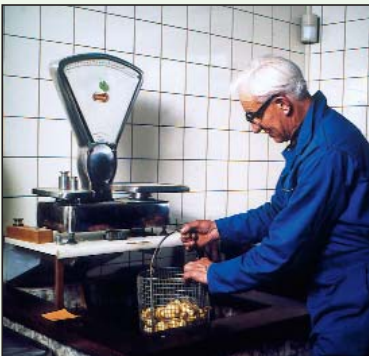
Determination of the weight in water of a potato sample
